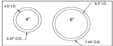
thin ring access plates feature fastenerless mounting, but may be drilled and counter bored for normal pan head screws or bolts.
